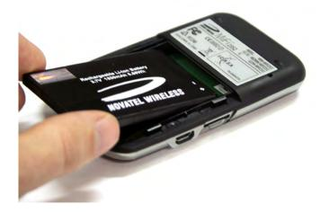
**4** Connect the wall charger to MiFi and charge for a minimum of 4 hours before use. The power button LED will flash amber while the device is charging and glow solid amber once charging is complete.
