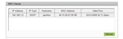
The WiFi Clients section of the WiFi Status page shows the clients that are currently connected to the MiFi. This is another way you can find the MAC address for a particular device when you are setting up MAC filtering.
