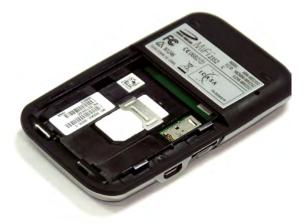
Now, insert the battery, lining up the contact points as shown and replace the door on the device.
